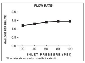
1.5 gpm/5.7 L/min. FLOW RATE
