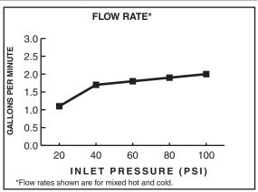
2.2 gpm/8.3 L/min. FLOW RATE
